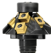
fig. 45°-bevel-milling head with 3x3 cutting edges and guide roller, equipped with 9 bevel-indexable inserts of type K
